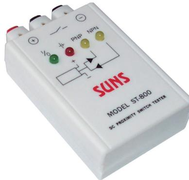
SUNS ST-800 proximity switch tester is designed to test most 3 wire DC proximity switches: inductives [metal sensing], capacitives, photoelectrics or ultrasonics. The unit is fitted with 2x 9V batteries ready for use.
